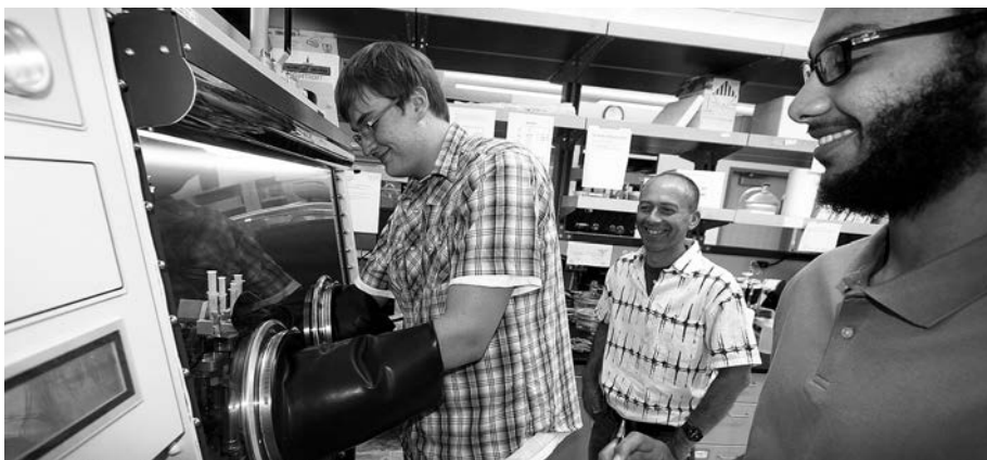
Chemistry-biochemistry students manipulate samples inside an airtight "glove box" in the lab with Colin Andrew, professor of chemistry.
